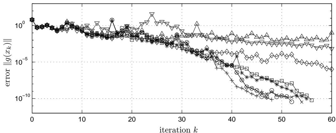
Figure 4: The convergence rate of the method of Broyden and the BRR method, for different values of  $p$ , applied to the period map of the reverse flow reactor using the one-dimensional model (4.1)-(4.3) with the parameter values of Table 2. [ $'o'$  (Broyden),  $'x'$  ( $p = 20$ ),  $'+'$  ( $p = 10$ ),  $'*'$  ( $p = 5$ ),  $'v'$  ( $p = 4$ ),  $'\diamond'$  ( $p = 3$ ),  $'\nabla'$  ( $p = 2$ ),  $'\triangle'$  ( $p = 1$ )]
