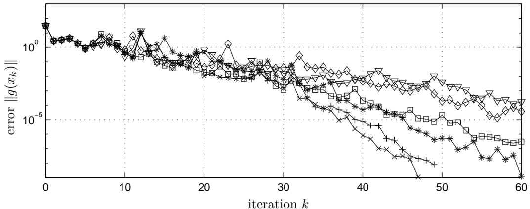
Figure 5: The convergence rate of the BRR method, for different values of  $p$ , applied to the period map of the reverse flow reactor using the two-dimensional model (4.5)-(4.7) with the parameter values of Tables 2 and 3. [ $\times$ ' ( $p = 20$ ),  $+$ ' ( $p = 10$ ),  $*$ ' ( $p = 5$ ),  $\square$ ' ( $p = 4$ ),  $\diamond$ ' ( $p = 3$ ),  $\nabla$ ' ( $p = 2$ )]
