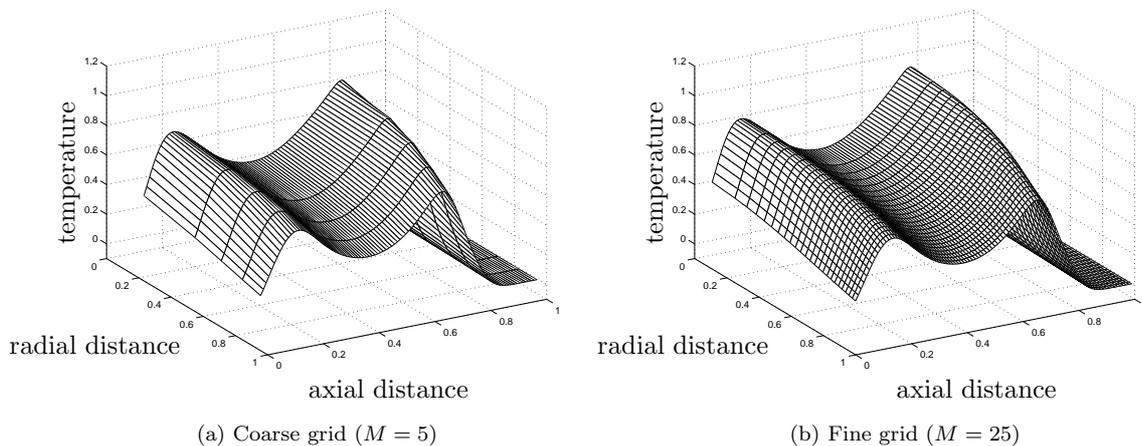
Figure 6: Temperature distribution over the reactor bed using a coarse and a fine grid.
