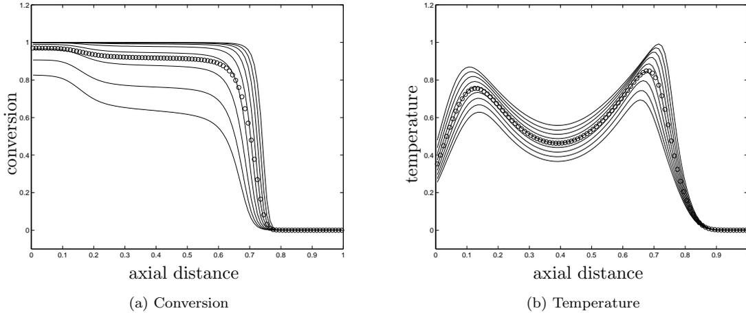
Figure 8: Axial temperature and conversion profiles of the RFR (in CSS) at the beginning of a reverse flow period using the two-dimensional model (4.5)-(4.7) with the parameter values of Tables 2 and 3. The cooling capacity  $\Phi$  is fixed at 0.2 and the radius of the reactor equals  $R/L = 0.025$ . In addition, the weighted average (4.9) is given ('o').
