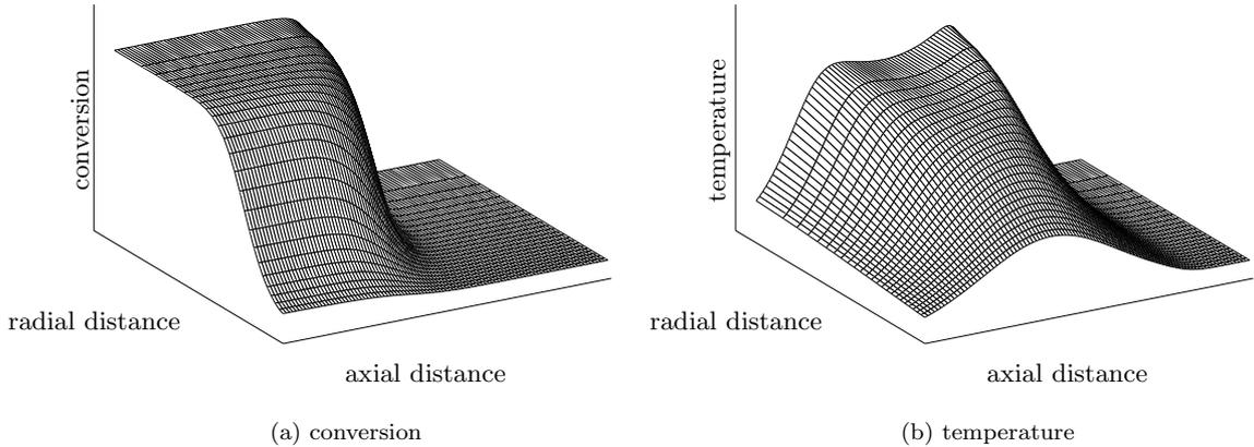
Figure 2: Qualitative temperature and conversion distribution of the cooled reverse flow reactor in the cyclic steady state using the two-dimensional model (4.5)-(4.7) with the parameter values of Tables 2 and 3.
