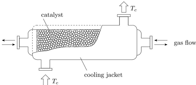
Figure 1: Schematic drawing of the cooled reverse flow reactor.
