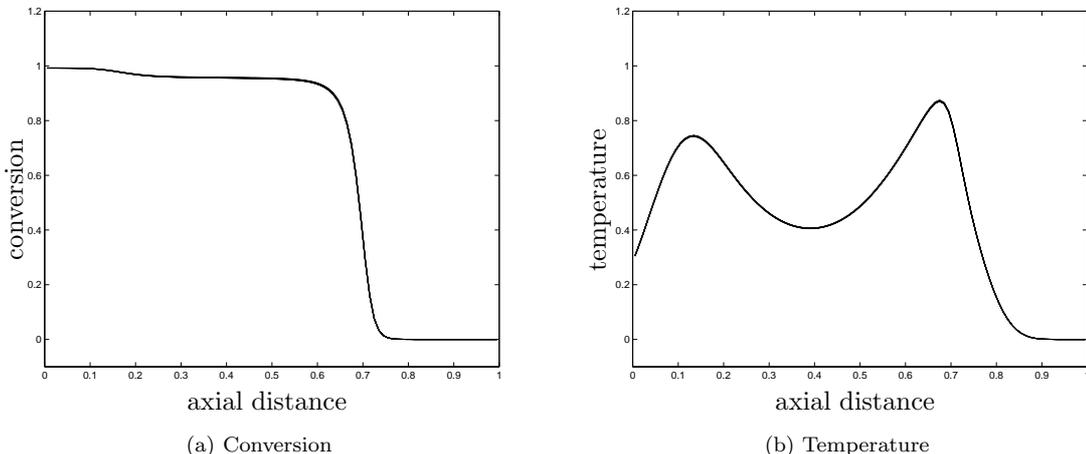
Figure 7: Axial temperature and conversion profiles of the RFR (in CSS) at the beginning of a reverse flow period using the two-dimensional model (4.5)-(4.7) with the parameter values of Tables 2 and 3. The cooling capacity  $\Phi$  is fixed at 0.2 and the radius of the reactor equals  $R/L = 0.0025$ .
