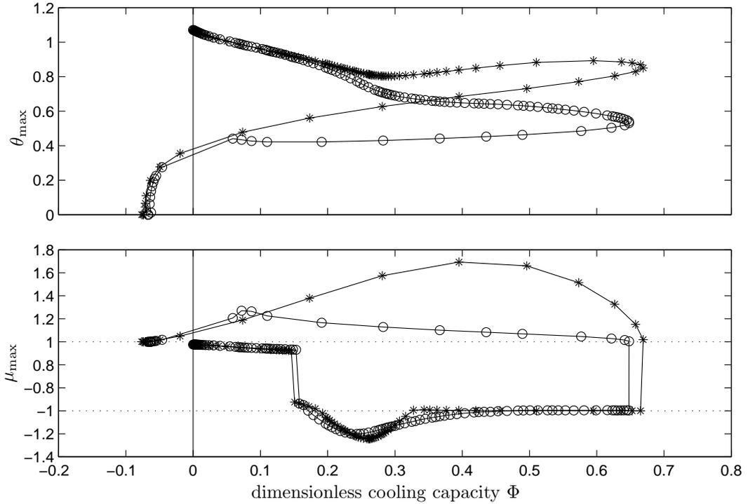
Figure 9: The maximum dimensionless temperature ( $\theta_{\max}$ ) and the largest Floquet multiplier ( $\mu_{\max}$ ) versus the cooling capacity ( $\Phi$ ) for two different values of the reactor radius. The two-dimensional model (4.5)-(4.7) was used with the parameter values of Tables 2 and 3. ['\*' ( $R/L = 0.0025$ ), 'o' ( $R = 0.025$ )]
